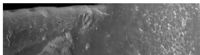
[Table/Fig-12]: SEM Analysis: Acrylic Liner shows an indistinct interface with sandblasted samples of denture base resin
